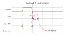
Other activations are corresponding to input mode 1 exept the *Loop Input* is inverted.
