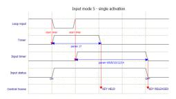
As illustrated above, a KEY HELD Central Scene notification will appear even though the activation on the input is shorter than configuration parameter 17. This is because the status on the input is prolonged with the time specified in the configuration parameter for the input timer (parameter 4/6/8/10/12/14).
