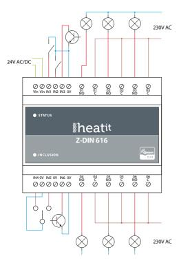
The Heatit Z-DIN 616 must be connected to a 24 Volt AC or DC power supply via the terminals labeled "Vin". The polarity is of no importance. The supply must be dimensioned to allow the supplied module with enough power to enable all relays to be activated. Regarding power consumption: see the technical details section.
