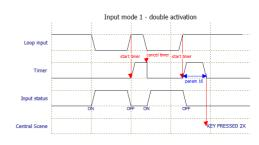
The figure above shows how a double activation is detected. The two activations must happen within the time specified in configuration parameter 16 to be accepted as a double activation.
