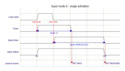
Other activations are corresponding to Input Mode 5, except the *Loop Input* is inverted.
