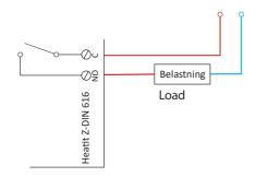
The 6 outputs of the Heatit Z-DIN 616 module consist of 1-pole SPST connectors (Single-Pole Single-Throw).
